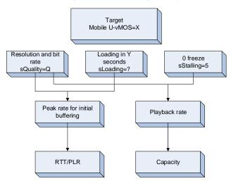
Figure 2-1 Basic process of network planning based on Mobile U-vMOS
